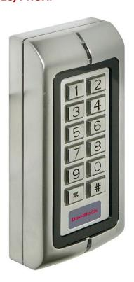
The range supports pin only, card only or a combination of pin and card operation with two relay outputs, lock and alarm. The keypad accepts a 125KHZ EM proximity card and uses two zones. Zone 1 offers up to 1100 Pin & Card holders and Zone 2 allows up to 100 Pin & Card holders.
