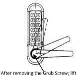
and rotate the lever handle 180 degrees anti-clockwise. Relocate the grub screw and tighten to secure lever handle
