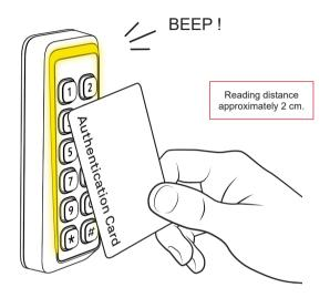
In order to set the reader in programming mode, present the valid "Authentication Card" to the reader as shown. The reader will beep and start blinking yellow to indicate that it is now in programming mode.
