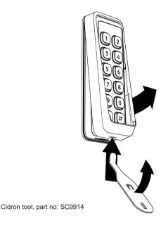
To open the reader, first remove the fixing screw and then detach the front cover from the installation plate by inserting the tip of the tool into the slot at the bottom of the front cover and move the tool upwards. This will release the front cover without damaging the front cover and/ or the installation plate.
