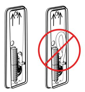
Make sure no excess connection cable is left in between the reader module and the installation plate.
