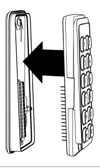
When installing the reader to the mounting plate ensure that the reader pin header contact perfectly aligns with the terminal connector block.
