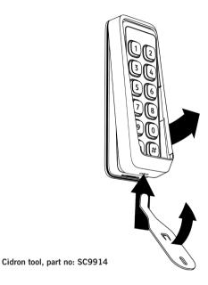
To open the reader, first remove the fixing screw and then detach the front cover from the installation plate by inserting the tip of the tool into the slot at the bottom of the front cover and move the tool upwards. This will release the front cover without damaging the front cover and/or the installation plate.
