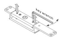
Using supplied key wrench to adjust armature plate to approx. 3 mm of gap between magnet and armeture.
