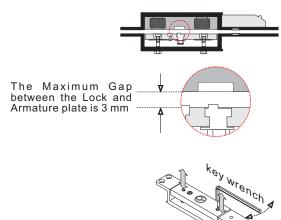
Using supplied key wrench to adjust armature plate to approx. 3 mm of gap between magnet and armature.
