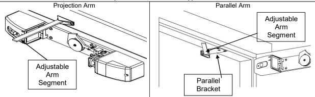
Configure the closer for left or right hand operation as appropriate (see the "Door Closer Configuration" section).
