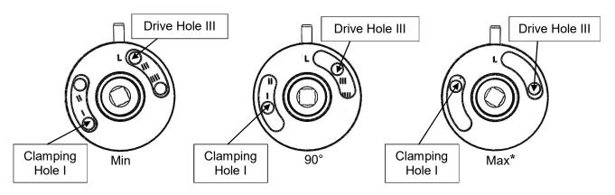
Figure 1: Left Hand Projecting Arm Cam Positions
