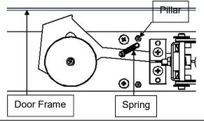
Separate the door closer arm and fit the adjustable arm segment to the door frame using 2 x  $N^{\circ}8$  \* 1-1/4"
