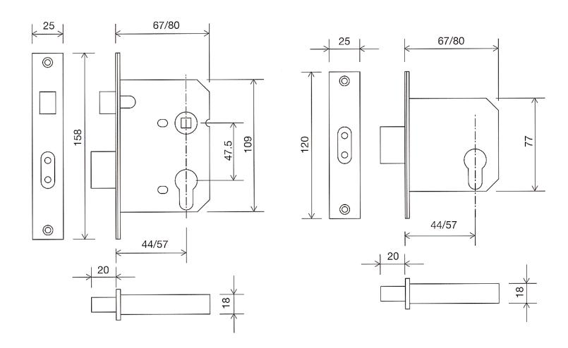
**UK manufactured High Security Euro Profile Mortice Sash & Dead Lock**
