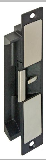
The AL990M series electric strikes are high in security and designed for use with all access control systems. The strikes are suitable for use with hinged doors which require security control as part of a building management system. These strikes are flexible and can be changed from fail safe to fail secure with the simple adjustment of the controlling screw and are available in 12 or 24V DC. They offer a strong, dependable and long-lasting electric strike solution.
