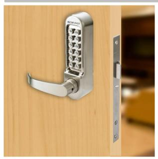
The unit includes a "Passage Mode" on the inside which is activated once a correct code is entered by turning a small turn. This allows the latch bolt to be engaged in the striker, but is withdrawn by either lever handle until the passage mode is released. Ideal for allowing a non-authorized person to come and go through the door when the door does not need to be secure.
