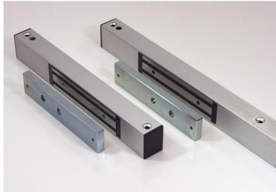
The AMG200 series mortice electromagnets are designed to offer a clean line across the door transom head or down the side door frame with the magnet encased into the satin anodised aluminium housing. Securefast Transom Housing has a high holding force of a nominal holding force of 600 lbf per magnet with different voltage options offering a sleek finish suitable for single or double outward door applications.
