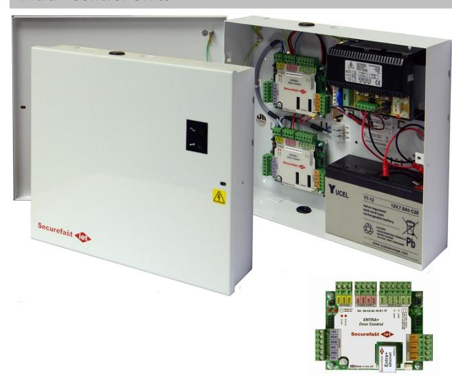
The Entra+ door controller supports all major reader types creating a total solution for your access control application. The controller has reader, RTE, door contact, auxiliary output and a 1.5A 12V lock output. The lock output may be changed on the board with a simple jumper from fail safe to fail secure.
