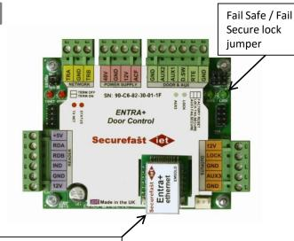
Additional plug-in Ethernet Adapter for connection to TCI/IP network.
