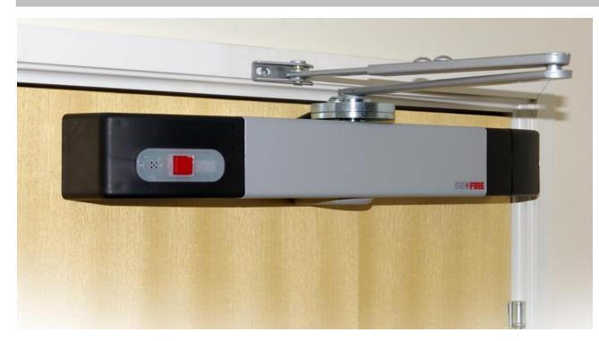
The Acoustic Door closer learns the sound of your specific fire alarm, releasing the door in the event of a fire. The closer is also battery operated so it can easily be retrofitted to any door. The AEM0070 door closer is ideally suited to environments such as care homes, schools and hospitals where it is essential to have doors in an open position at certain times of the day to aid access, but equally as important to ensure the doors are closed in the event of a fire.
