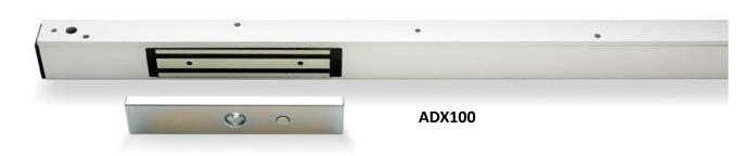
The Deedlock Slimline Mortice Electro Magnetic Lock have 600lb holding force and is mounted in a transom housing offering a visually improved appearance. Securefast Slimline Magnet is ideal for use with the panic exit hardware where a delayed egress is required. Continuous housing provides an improved aesthetics for high quality installations
