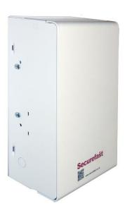
The Securefast ADP324-FR power supply unit is a small case 24V DC switched-mode 500mA power supply specially designed to power magnetic fire alarm door retainers and general 24 Volt DC applications.
