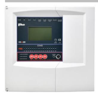
The CIE-A-200 Addressable Fire Alarm Control Panel is a one loop panel capable of supporting up to 200 devices with a maximum loop length of 2km, the panel also provides two configurable monitored input circuits, 2 configurable monitored output circuits, 2 configurable + 1 fault relay and also a Peripheral bus circuit to add up to 8 repeater panels.
